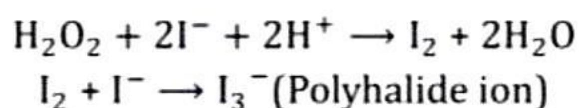
The reaction is monitored by adding a known volume of sodium thiosulphate solution and starch solution to the reaction mixture. Iodine liberated at once reacts with thiosulphate solution and is reduced to iodide ions:
