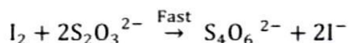
When thiosulphate ions are completely consumed, the liberated iodine reacts with starch solution and gives blue colour.
